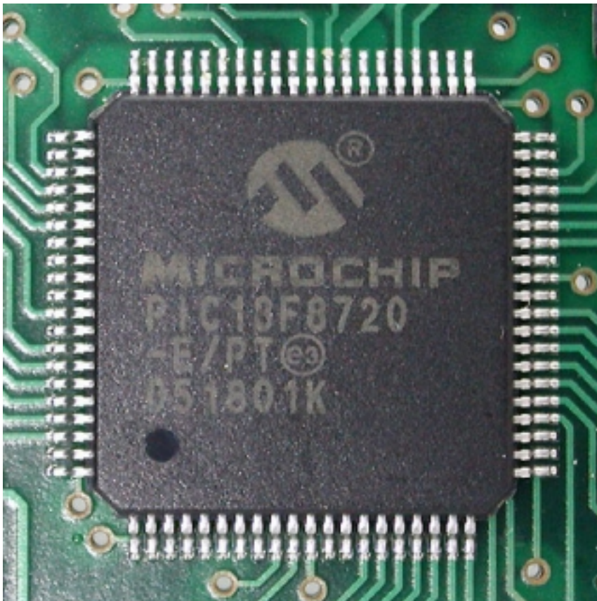
A PIC 18F8720 microcontroller
